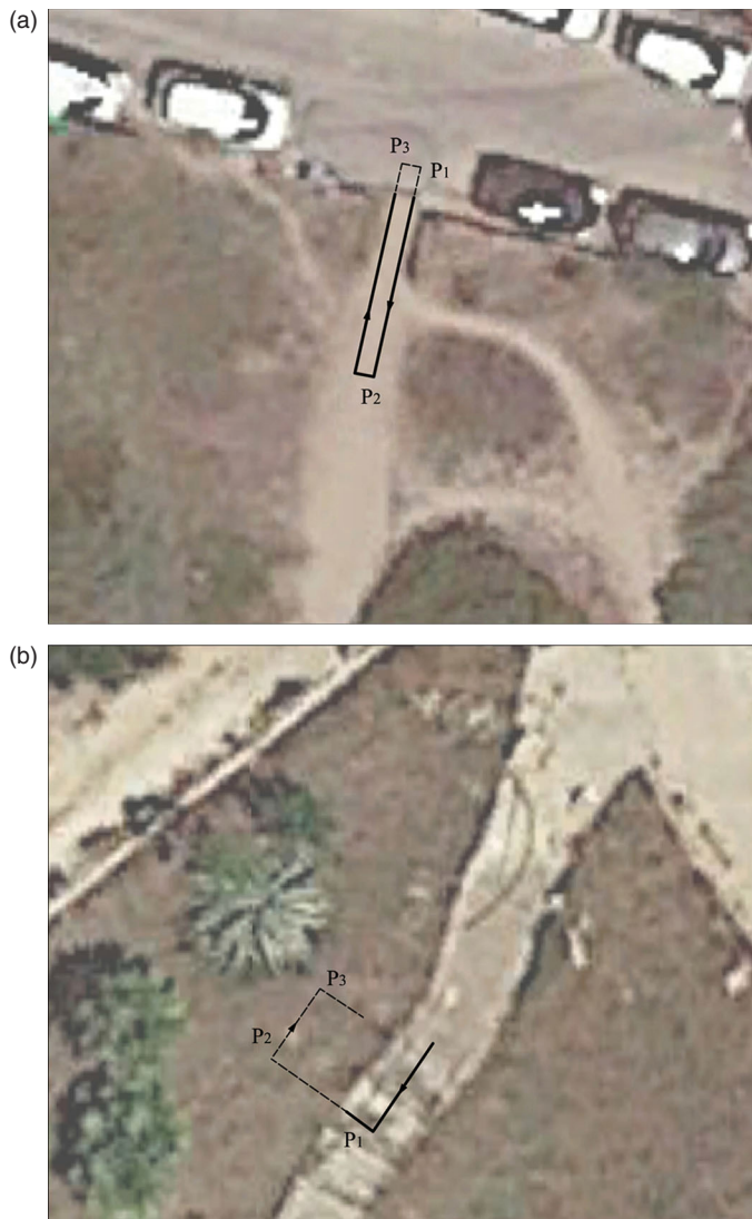
Figure 13. Field experiments along mixed-terrain paths to validate the proposed terrain classifier: (a) asphalt and sand ( 39^{\circ}51'3.30''\text{N} , 18^{\circ}10'50.98''\text{E} ), and (b) dirt road and plowed terrain ( 40^{\circ}3'35.08''\text{N} , 18^{\circ}20'42.57''\text{E} ). Please refer to Table 5 for classification results.
