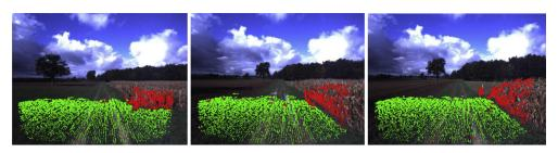
Fig. 4 – Results obtained from the geometry-based classifier in a maize crop. Green dots denote ground-labelled points, red dots denote points classified as non-ground.
