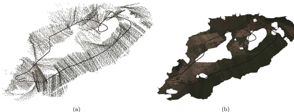
**Figure 17.** (a) Radar-generated map, shown as raw data obtained from the classifier with associated RGB data obtained from the visual classifier. (b) Same radar-vision data after Delaunay triangulation.
