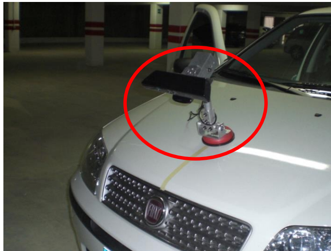
Fig. 1 The experimental test bed equipped with a Microsoft Kinect camera for parking assistance purposes
