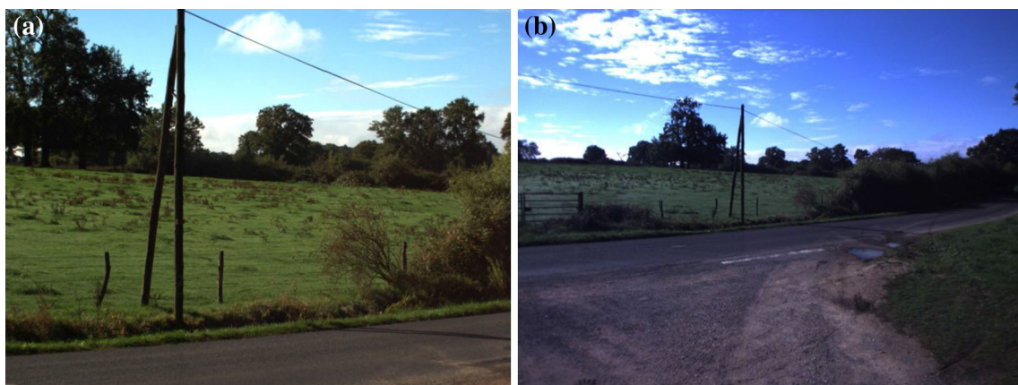
Fig. 4 Sample images acquired during experimentation by the Flea3 system (a) and the XB3 system (b). It can be noted that the angular field of view of the XB3 is wider than the one of the Flea3 due to the use of a shorter focal length. However, the Flea3 image displays more clearly far away objects
