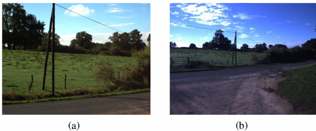
Fig. 4: Sample images acquired during experimentation by the Flea3 system (a) and the XB3 system (b). It can be noticed that the angular field of view of the XB3 is wider than the one of the Flea3 due to the use of a shorter focal length. However, the Flea3 image displays more clearly far away objects.
