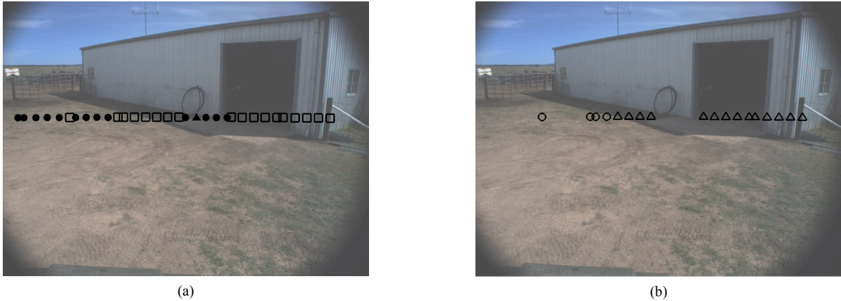
Fig. 4. (a) Observations obtained by the radar at scan #778 before visual classification. Black dots and triangles denote radar-labeled ground and non-ground observations, respectively. Outlined squares denote uncertain measurements. (b) Results after classification of the unknowns using the visual classifier. Outlined circles and triangles denote ground and non-ground, respectively.
